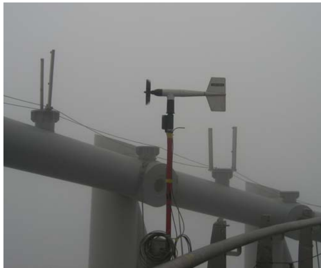
Fig. 3 Anemometer at top of the main tower ( z = 461.1 m)
