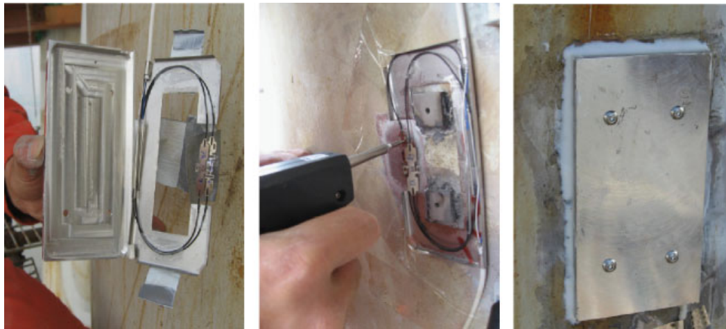
Figure 13. Installation and protection of FBG sensor.
